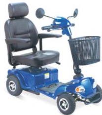
TC141 Comfortable SwivelSeat,Flip-Up Armrest, Driving Lamp And Luggage Basket. Rubber Foam Castor Rubber Foam Rear Wheel.
